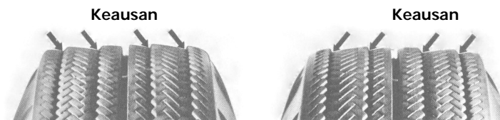
Gambar 31. Keausan Ban Akibat Toe – out
